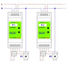
The descriptions of the screw terminals are printed on the adapter label. The "O1" and "O2" letters indicate the relays outputs.
