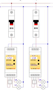
The descriptions of the screw terminals are printed on the adapter label. The "O1" and "O2" letters indicate the relays outputs.
